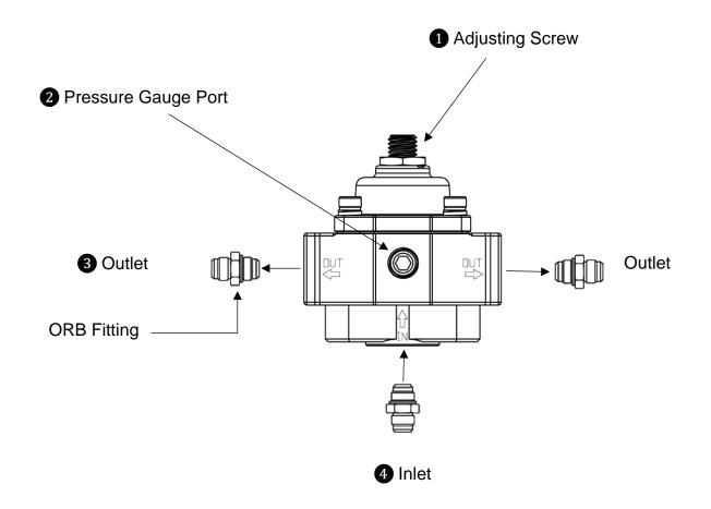
**1** The regulator is designed with a threaded adjuster and locking nut at the top which alters the preload on the internal spring. Increasing the preload will increase the fuel pressure.
